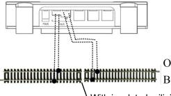
Connecting to the track - ensure that O and B from both outputs are connected to the same rail
